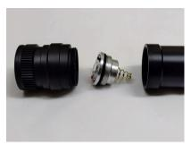
Fit the o-ring to the pill behind the shoulder to space the pill closer to the lens.
